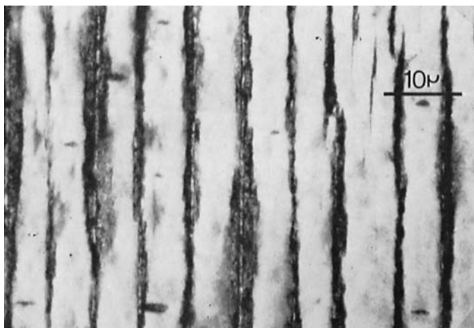
Fig. 9. Surface of specimen of polyethylene sheet after treatment with fuming nitric acid at 60°C for 5 hr showing cracks perpendicular to the draw direction (the draw direction is parallel to the length marker).
